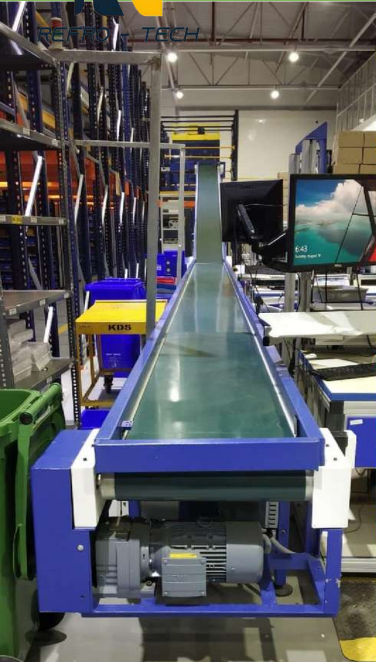
Inclined belt conveyor connecting ground level
