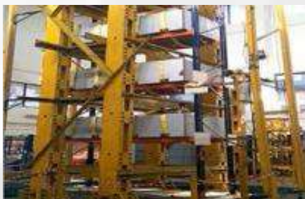
Safety in design – Tested Seismic racking for zone 5 and above
