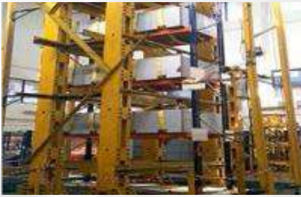
Safety in design – Tested Seismic racking for zone 5 and above
